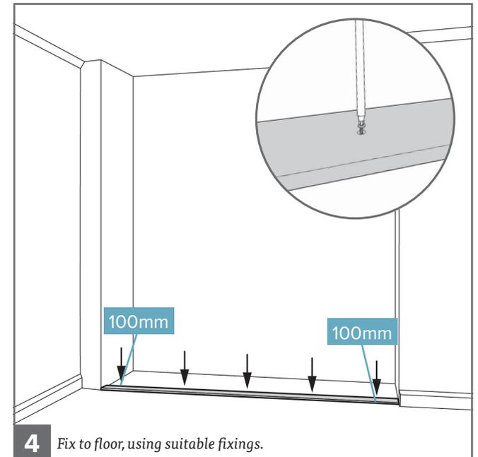
**4** Fix to floor, using suitable fixings.
