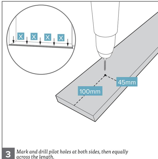
**3** Mark and drill pilot holes at both sides, then equally across the length.
