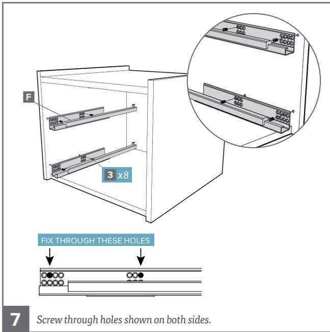
**7** Screw through holes shown on both sides.
