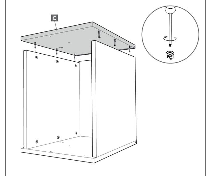
**6** Push/tap into place and tighten the cam locks.
