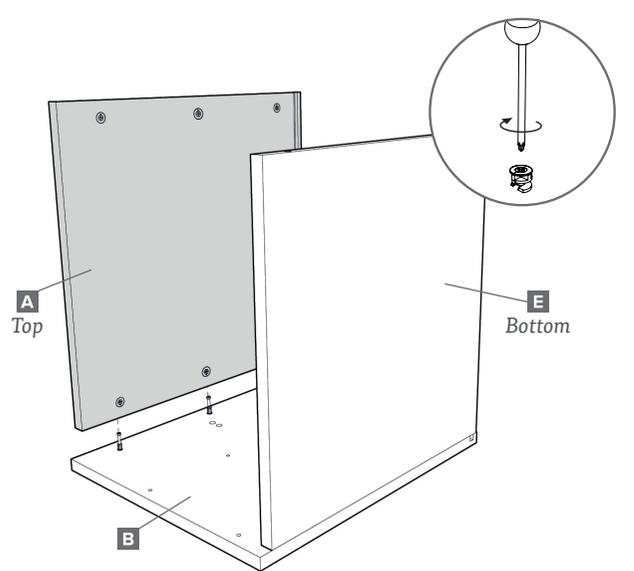
**4** Push/tap into place and tighten the cam locks.
